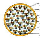
LSOH (SHF1) Outer Sheath Tinned Copper Drain Wire XLPE Insulation Al/polyester Tape Screen Mica Glass Tape Stranded Copper Conductor
